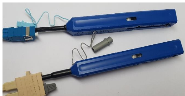
Cleaning tools with adaptor removed and the tip in a through adaptor for cleaning internal connector or a Fibre port requiring cleaning
