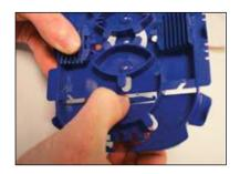
To remove fiber pick press down firmly on pick before mounting tray.
