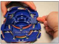
Use finger nail or tapered end of fiber cutouts and flex lid up at center pivot upwards.
