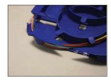
Routing underneath splice holder area
