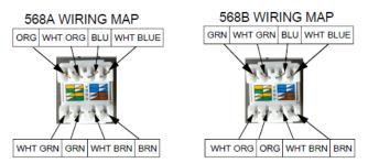
**b)** Terminate the cable with a 110 Termination tool ensuring the cable sheath is maintained to the base of the IDC towers and allowing a maximum untwist of 6mm.
