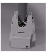
**d)** Important: To achieve optimum alien cross talk prevention, place the IDC cap cover the IDC towers. Align the "UP" mark on the cap with the "UP" mark on the jack latch. Snap the cap into place to ensure fully seated.
