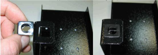
3.3) Install half of the Finger Guide at the top and end of 19" Vertical Rack Manager. Fasten it with a screw delivered in a kit. Use electric screwdriver for quick and comfortable installation.
