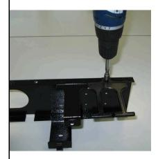
3.4) Install 8 Finger Guides at the middle of 19" Vertical Rack Manager. Fasten it with a screws delivered in a kit. Use electric screwdriver for quick and comfortable installation.
