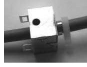
6c. Remove 3 of the 4 foils from the cable pairs. Unwrap the foil from 1 pair in preparation for Wrapping around the cable sheath.
