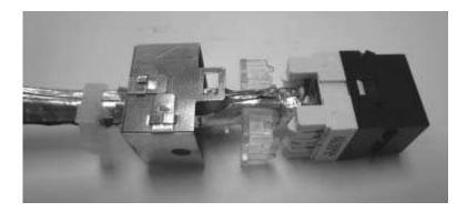
2k. Ensure cables are trimmed off flush with IDC, if not use side cutters to remove excess cable after termination.
