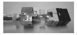
6j. Ensure cables are trimmed off flush with IDC, if not use side cutters to remove excess cable after termination.
