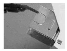
2e. Remove 100mm of cable sheath. Cut central separator back to sheath. Cut cellophane wrap back to sheath. Wrap foil around cable.
