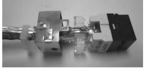
Ensure cables are trimmed off flush with IDC, if not use side cutters to remove excess cable after termination.
