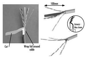
2f. Wrap drain wire around foil and tighten, leaving a length of drain wire available for wrapping around rear can cable clamp.
