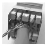
4f. Ensure cables are trimmed off flush with IDC, if not use side cutters to remove excess cable after termination.
